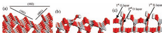
Figure 1. Structures of anatase surfaces: (a) overview of anatase (101), (001), and (102) surfaces; (b) anatase (101) with H 2 O adsorption; and (c) anatase (001) with half a monolayer of dissociated H 2 O. Ti, gray; O, red; H, white.
